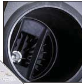
Melt tank with dual pre-melt grids.
