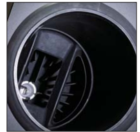
Melt tank with dual pre-melt grids.
